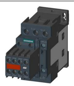
CONTACTOR, AC-3, 11KW/400V, 2NO+2NC, AC 110V 50HZ 120V 60HZ, W. PLUGGED-IN VARISTOR 3POLE, SZ. SO SCREW TERMINAL
