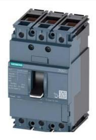
CIRCUIT BREAKER 3VA1 IEC FRAME 160 BREAKING CAPACITY CLASS H ICU=70KA @ 415 V 3-POLE, LINE PROTECTION TM210, FTFM, IN=40A OVERLOAD PROTECTION IR=40A FIXED SHORT CIRCUIT PROTECTION II=10 X IN CABLE CONNECTION
