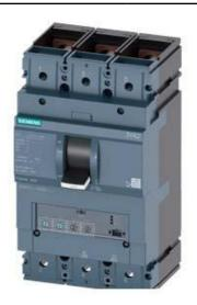
CIRCUIT BREAKER 3VA2 IEC FRAME 400 BREAKING CAPACITY CLASS C ICU=110KA @ 415 V 3-POLE, LINE PROTECTION ETU350, LSI, IN=250A OVERLOAD PROTECTION IR=100A ...250A SHORT CIRCUIT PROTECTION ISD=1,5... 10 X IR, II=12 X IN BUSBAR CONNECTION
