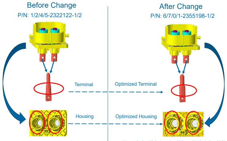
端子和塑壳形状有变,成品外部尺寸没有变化,性能没有变化 Only terminal and housing changed, but no other change, no performance change.
