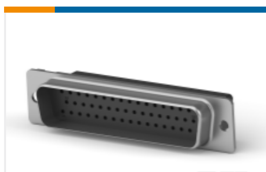
TE Part #1658641-2 D-Sub Crimp: Plug, Signal, 50 Posn, Pin Size 20, Shell Size 5
