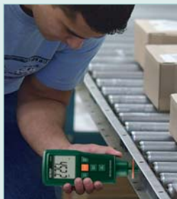
Contact Tachometer function measures the speed of rotating objects by placing the wheel tip onto the surface.
