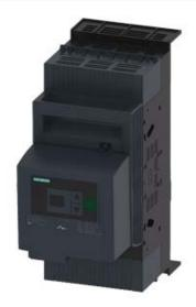
FUSE-SWITCH-DISCONNECTOR 3-POLE, NH000, 160A 40MM BUSBAR SYSTEM COVER LEVEL 32/70 MM BOX TERMINAL FUSE MONITORING ELECTRONIC, EFM 20
