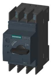
CIRCUIT-BREAKER SZ S00, FOR MOTOR PROTECTION, CLASS 10, A-RELEASE 0.11...0.16A, N-RELEASE2.1A RING CABLE LUG CONNECTION STANDARD SW. CAPACITY
