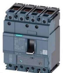
CIRCUIT BREAKER 3VA1 IEC FRAME 160 BREAKING CAPACITY CLASS M ICU=55KA @ 415 V 4-POLE, LINE PROTECTION TM240, ATAM, IN=125A OVERLOAD PROTECTION IR=87,5A ...125A SHORT CIRCUIT PROTECTION II=5...10 X IN NEUTRAL UNPROTECTED CABLE CONNECTION
