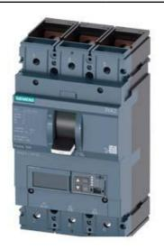
CIRCUIT BREAKER 3VA2 IEC FRAME 630 BREAKING CAPACITY CLASS H ICU=85KA @ 415 V 3-POLE, LINE PROTECTION ETU850, LSI, IN=400A OVERLOAD PROTECTION IR=160A ...400A SHORT CIRCUIT PROTECTION ISD=0,6..10X IN, II=1,5..15X IN NEUTRAL PROTECTION OPTIONAL WITH EXT. CT;UPTO 160% BUSBAR CONNECTION
