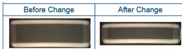
Image 2. Cross section of MLCC before and after dielectric thickness change
