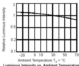
Luminous Intensity vs. Ambient Temperature
