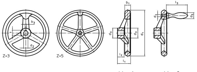
The orientation of the hub keyway may be different than shown in the drawing.
