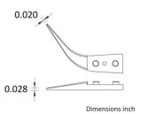
**Tip dimensions:** Tip width 0.50 mm - 0.020 inch Tip thickness 0.70 mm - 0.028 inch
