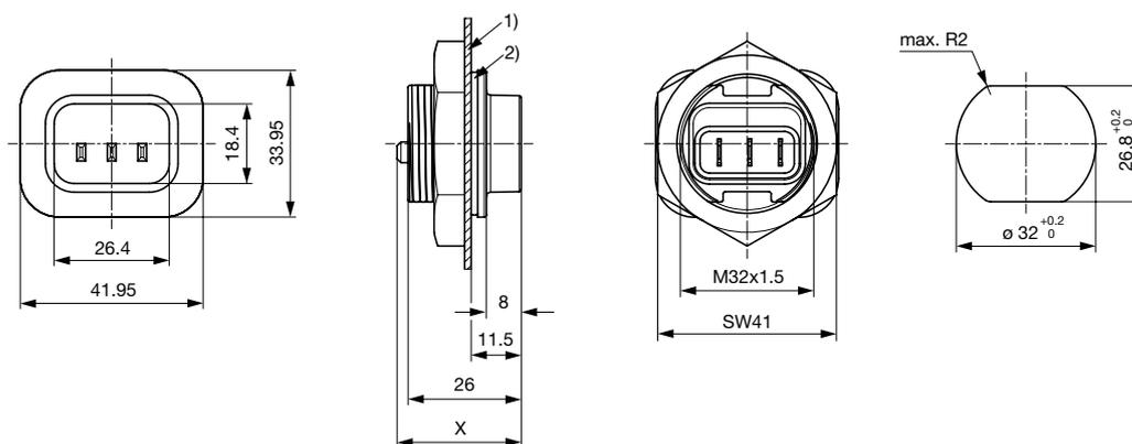
X: Steckanschlüsse 4.8x0.8 mm: 28.5 mm
