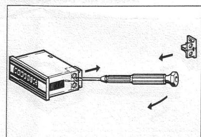
For the universal terminal remove the cap by lightly turning or prising with the screwdriver. Then take out the screw and the screw terminal becomes an AMP terminal.
