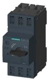
CIRCUIT-BREAKER SZ S00, FOR TRANSFORMER PROT. A-RELEASE 5.5...8A, N-RELEASE 163A, SPRING-L. CONNECTION, STANDARD SW. CAPACITY
