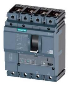
CIRCUIT BREAKER 3VA2 IEC FRAME 160 BREAKING CAPACITY CLASS M ICU=55KA @ 415 V 4POLE, LINE PROTECTION ETU320, LI, IN=100A OVERLOAD PROTECTION IR=40A ...100A SHORT CIRCUIT PROTECTION II=12 X IN NEUTRAL PROTECTION ADJUSTABLE(OFF,50%,100%) BUSBAR CONNECTION
