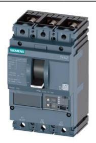
CIRCUIT BREAKER 3VA2 IEC FRAME 250 BREAKING CAPACITY CLASS C ICU=110KA @ 415 V 3POLE, LINE PROTECTION ETU860, LSIG, IN=250A OVERLOAD PROTECTION IR=100A ...250A SHORT CIRCUIT PROTECTION ISD=0,6..10X IN, II=1,5..10X IN NEUTRAL PROTECTION OPTIONAL WITH EXT. CT,UPTO 160% GROUNDFAULT, SWITCHABLE IG=0,2... 1 X IN, TG=0,050,8MS BUSBAR CONNECTION
