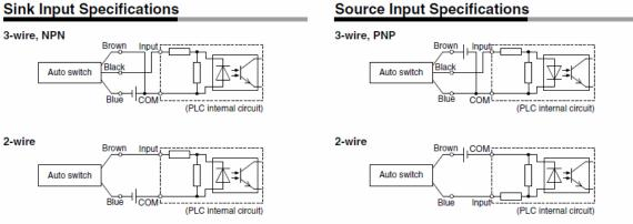
Connect according to the applicable PLC input specifications, as the connection method will vary depending on the PLC input specifications.
