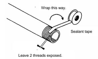
Fig. 2 Sealant tape
