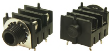
FCR1210WMN - S2S/BNB/PCC/WM/N/FW MONO JACK SOCKET WITH PC LEGS AND FITTED EARTH WASHER WITH 1 PC LEG SUPPLIED WITH FIBRE WASHER AND BLACK PLASTIC NUT
