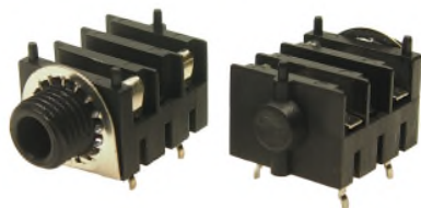
FCR1210W - S2S/BNB/PCC/EW/N MONO JACK SOCKET WITH PC LEGS AND FITTED EARTH WASHER WITH 2 PC LEGS SUPPLIED WITH BLACK PLASTIC NUT
