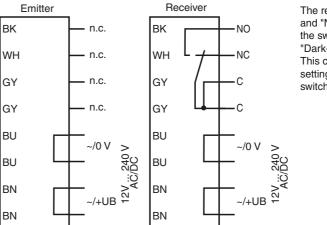
The relay-functions "NC" and "NO" bear on the switching mode "Dark-ON". This complies to the default setting of the light/dark switch (factory setting).
