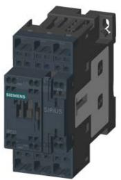
CONTACTOR, AC-3, 15KW/400V, 1NO+1NC, AC(50-60HZ)/DC ACTUAT. AC/DC 95...130V, 3-POLE, SZ S0 SPRING-LOADED TERMINAL
