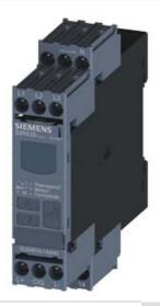
DIGITAL MONITORING RELAY FOR THREE-PHASE LINE VOLTAGE FOR IO-LINK AC 50 TO 60 HZ 3X 160 TO 690V LINE PHASE SEQUENCE, PHASE FAILURE, PHASE ASYMMETRY UNDER- AND OVERVOLTAGE HYSTERESIS 1-20V NETWORK STABILITY TIME TRIGGER DELAY TIME 1 CO CONTACT, SCREW TERMINAL
