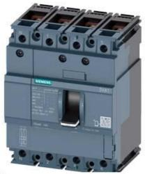
CIRCUIT BREAKER 3VA1 IEC FRAME 160 BREAKING CAPACITY CLASS M ICU=55KA @ 415 V 4-POLE, LINE PROTECTION TM210, FTFM, IN=50A OVERLOAD PROTECTION IR=50A FIXED SHORT CIRCUIT PROTECTION II=10 X IN NEUTRAL UNPROTECTED BUSBAR CONNECTION
