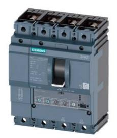
CIRCUIT BREAKER 3VA2 IEC FRAME 100 BREAKING CAPACITY CLASS C ICU=110KA @ 415 V 4POLE, LINE PROTECTION ETU330, LIG, IN=63A OVERLOAD PROTECTION IR=25A ...63A SHORT CIRCUIT PROTECTION II=1,5...12 X IN NEUTRAL PROTECTION ADJUSTABLE(OFF,100%) GROUNDFAULTPROTECTION IG=0,2... 1 X IN, TG=0,1/0,3MS BUSBAR CONNECTION
