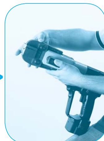
Lock in position by closing the retaining pin.
