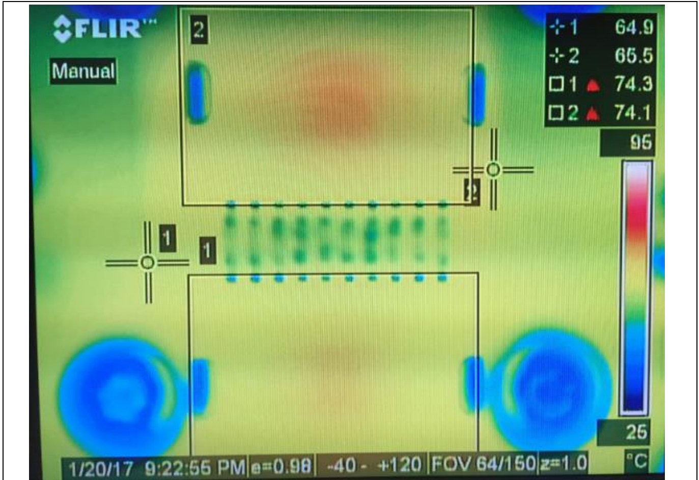
Figure 9 Temperature measurement of GaN devices at full load (2500 W, 230 V AC input)
