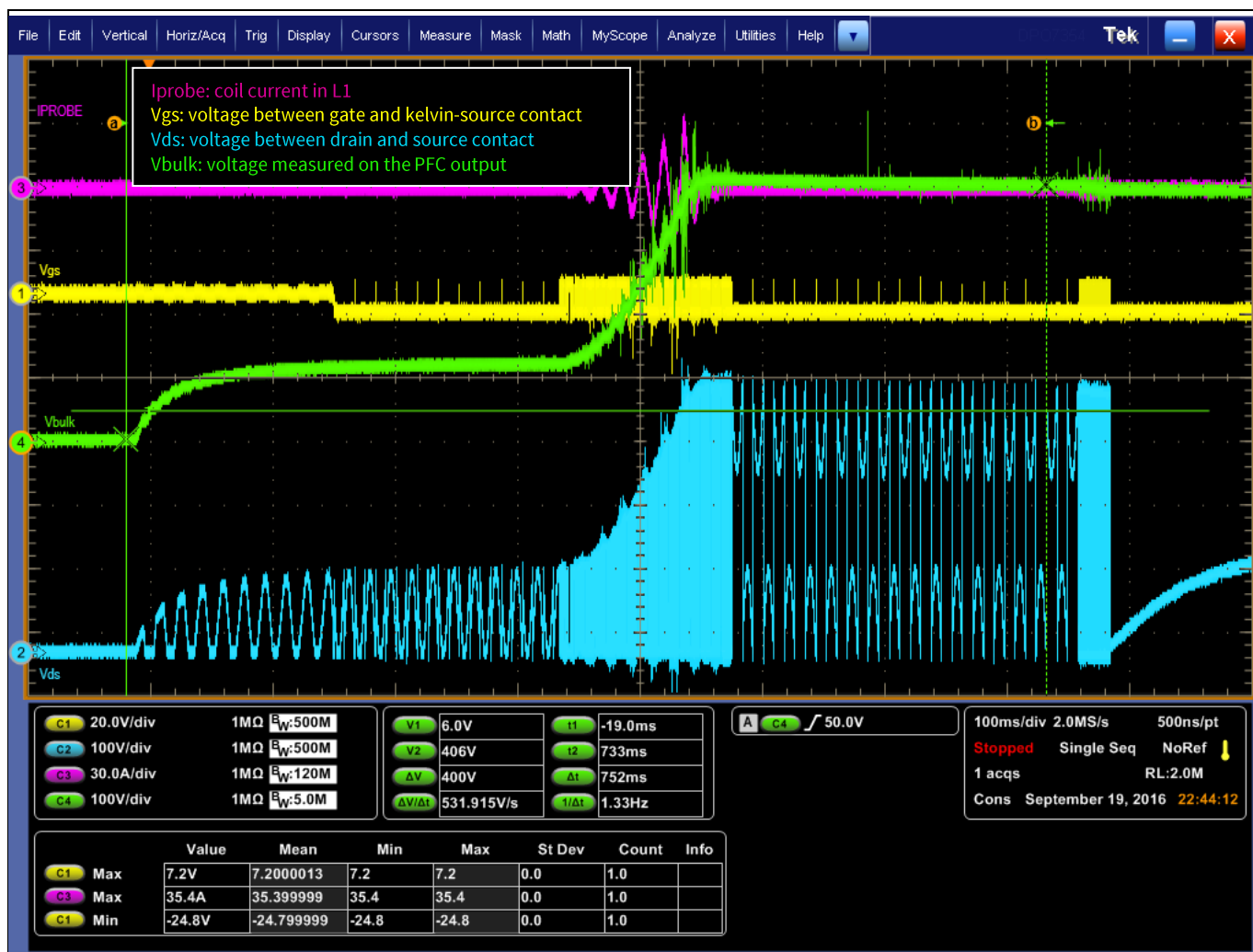
Figure 31 Start-up of PFC at 90 V rms without load current. The blue curve represents the V DS voltage, the magenta curve shows the input current, the green curve shows the DC-link voltage and the yellow curve shows the V GS voltage of the GaN HEMT. The measured peak input current is 35.4 A.
