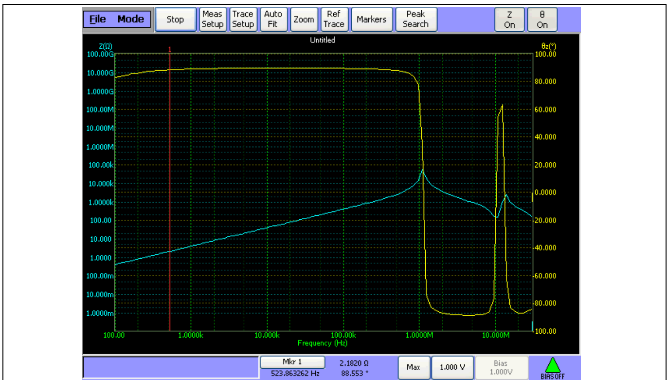
Figure 3 Frequency sweep of PFC coil showing inductive behavior over a wide range and the first resonance above 1 MHz
