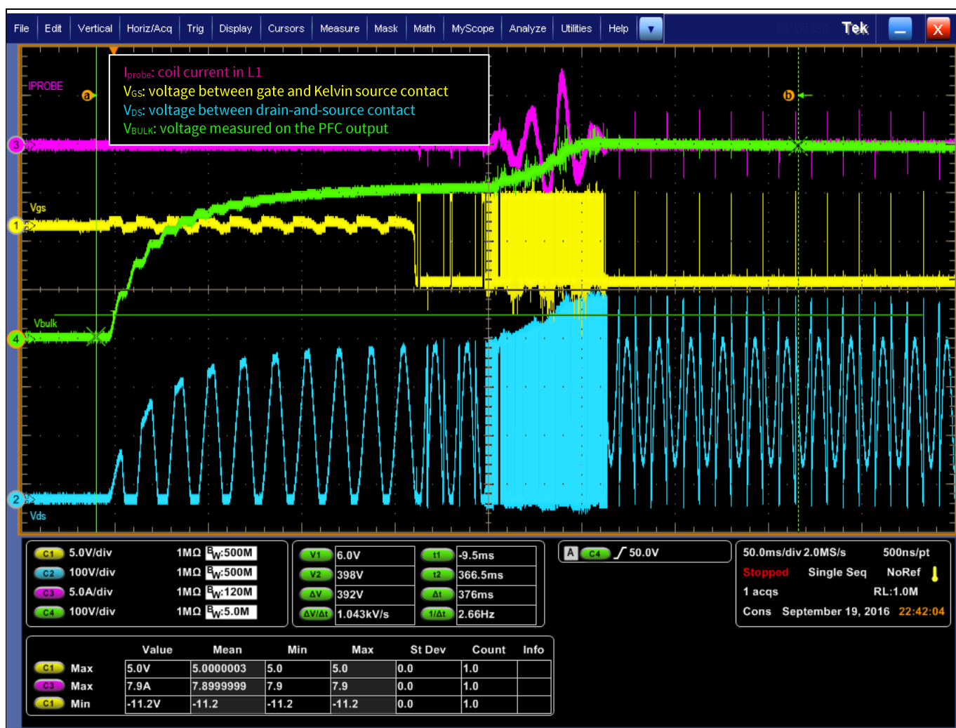
Figure 30 Start-up of PFC at 230 V rms without load current. The blue curve represents V DS voltage, the magenta curve shows the input current, the green curve shows the DC link voltage and the yellow curve shows V GS voltage of the GaN HEMT. The measured peak input current is 7.9 A.
