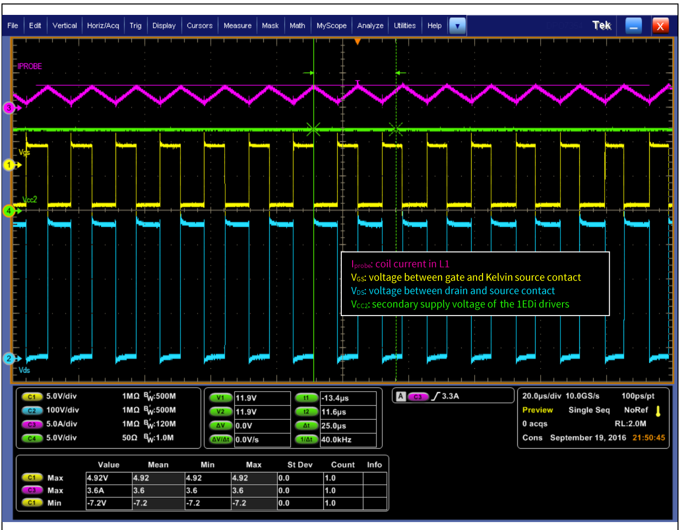
Figure 33 Continuous operation at nominal conditions ( V_{in} = 230 V_{rms} ); the output power is 500 W. The blue curve represents V_{DS} , the magenta curve shows the input current, the green curve shows the supply voltage of the 1EDi drivers on the secondary side and the yellow curve shows V_{GS} voltage of the GaN HEMT.
