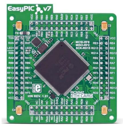
PIC32MZ2048EFH144 - a 32-bit MCU with 512 KB of SRAM and 2MB of Flash, 250MHz maximum frequency, an internal oscillator, audio and graphic interfaces, Ethernet and more.
