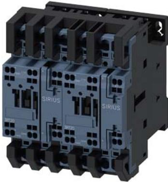
Wendekombination AC-3, 11 kW/400 V AC 110 V 50Hz/120V 60Hz,3-polig
