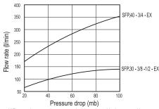
(difference between the pressure inside and outside the reservoir) SFP+F FOAM-EX
