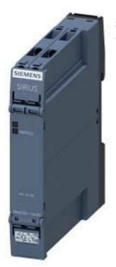
Thermistor motor prot. relay Compact evaluation unit 17.5 mm enclosure Screw terminals 1 CO contact US = 24 V AC/DC Auto RESET Suitable for bimetal switches Supply = output voltage 1 LED (READY)
