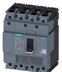
CIRCUIT BREAKER 3VA1 IEC FRAME 160 BREAKING CAPACITY CLASS M ICU=55KA @ 415 V 4-POLE, LINE PROTECTION TM220, ATFM, IN=16A OVERLOAD PROTECTION IR=11,2A ... 16A SHORT CIRCUIT PROTECTION II=10 X IN NEUTRAL PROTECTION 100% BUSBAR CONNECTION
