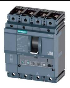
CIRCUIT BREAKER 3VA2 IEC FRAME 160 BREAKING CAPACITY CLASS H ICU=85KA @ 415 V 4POLE, LINE PROTECTION ETU350, LSI, IN=100A OVERLOAD PROTECTION IR=40A ...100A SHORT CIRCUIT PROTECTION ISD=1,5... 10 X IR, II=12 X IN NEUTRAL PROTECTION ADJUSTABLE(OFF,50%,100%) BUSBAR CONNECTION
