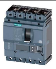
CIRCUIT BREAKER 3VA2 IEC FRAME 160 BREAKING CAPACITY CLASS H ICU=85KA @ 415 V 4POLE, LINE PROTECTION ETU860, LSIG, IN=160A OVERLOAD PROTECTION IR=64A ...160A SHORT CIRCUIT PROTECTION ISD=0,6..10X IN, II=1,5..10X IN NEUTRAL PROTECTION ADJUSTABLE (OFF, UPTO 100%) GROUNDFAULT, SWITCHABLE IG=0,2... 1 X IN, TG=0,050,8MS BUSBAR CONNECTION
