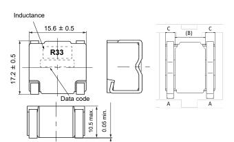
※ The mounting terminal should not protrude from C
