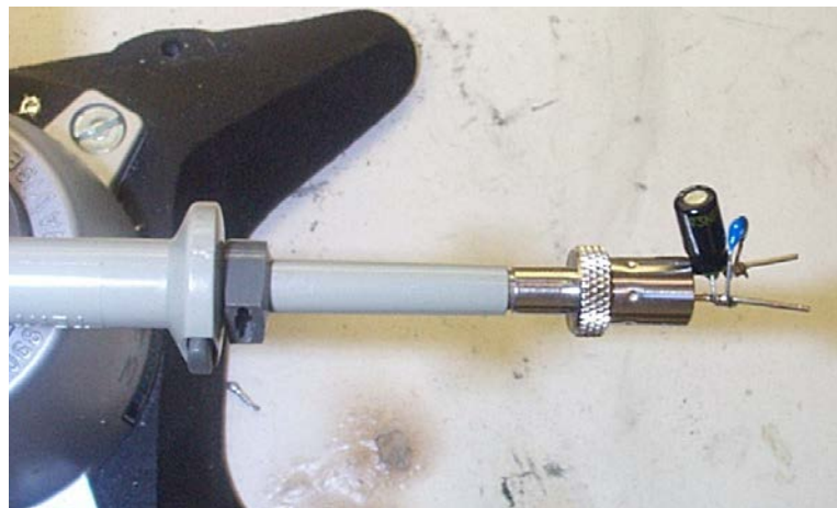
Figure 45 – Oscilloscope Probe with Probe Master ( www.probemaster.com ) 4987A BNC Adapter. (Modified with wires for ripple measurement, and two parallel decoupling capacitors added)
