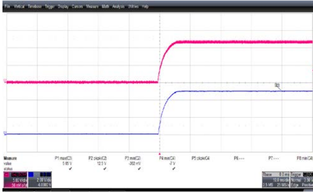
Figure 36 – Output Voltage and Current Waveforms. 85 VAC Input. Upper: 5 V, 2 V / div. Middle: I_{OUT} , 1 A / div. Lower: 12 V, 5 V, 1.6 ms / div.
