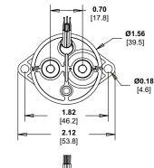
MOUNTING - 2 PLCS (HARDWARE NOT SUPPLIED) 2 X M4 BOLT, LOCKWASHER AND WASHER TORQUE: 20 IN-LBS (2.3 NM) MAX
