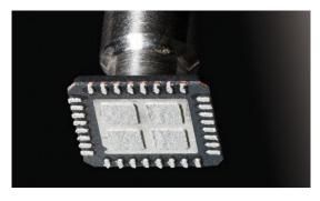
MLF 32 with solder paste printed on the bottom
