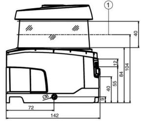
Part no.: 53800261 – RSL440-L/CU429-300-WPU – Safety laser scanner
