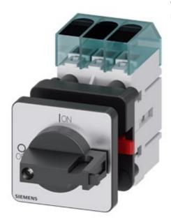
Switch disconnector 3LD3, main switch 3-polig, Iu 32A operational switch at AC-23 A at 400 V 11,5 kW front mounted Base mounting with center-hole 22,5 mm knob-operated mechanism black 48 x 48 mm
