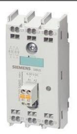
SOLID STATE RELAY 3-PHASE 3RF2 30 A 40 DEG. C 48-600 V / 4-30 V DC 3PH.-CONTROLLED SPRING-TYPE TERMINALS BLOCKING VOLTAGE 1200 V
