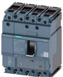
CIRCUIT BREAKER 3VA1 IEC FRAME 160 BREAKING CAPACITY CLASS N ICU=25KA @ 415 V 4-POLE, LINE PROTECTION TM240, ATAM, IN=125A OVERLOAD PROTECTION IR=87,5A ...125A SHORT CIRCUIT PROTECTION II=5...10 X IN NEUTRAL PROTECTION 50% CABLE CONNECTION
