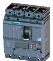
CIRCUIT BREAKER 3VA2 IEC FRAME 100 BREAKING CAPACITY CLASS L ICU=150KA @ 415 V 4POLE, LINE PROTECTION ETU550, LSI, IN=25A OVERLOAD PROTECTION IR=10A ...25A SHORT CIRCUIT PROTECTION ISD=0,6..10X IN, II=1,5..12X IN NEUTRAL PROTECTION ADJUSTABLE (OFF, UPTO 160%) BUSBAR CONNECTION
