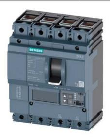
CIRCUIT BREAKER 3VA2 IEC FRAME 160 BREAKING CAPACITY CLASS C ICU=110KA @ 415 V 4POLE, LINE PROTECTION ETU560, LSIG, IN=40A OVERLOAD PROTECTION IR=16A ...40A SHORT CIRCUIT PROTECTION ISD=0,6..10X IN, II=1,5..12X IN NEUTRAL PROTECTION ADJUSTABLE (OFF, UPTO 160%) GROUNDFAULT, SWITCHABLE IG=0,2... 1 X IN, TG=0,050,8MS CABLE CONNECTION
