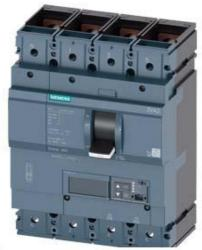
CIRCUIT BREAKER 3VA2 IEC FRAME 400 BREAKING CAPACITY CLASS H ICU=85KA @ 415 V 4-POLE, LINE PROTECTION ETU550, LSI, IN=250A OVERLOAD PROTECTION IR=100A ...250A SHORT CIRCUIT PROTECTION ISD=0,6..10X IN, II=1,5..12X IN NEUTRAL PROTECTION ADJUSTABLE (OFF, UPTO 160%) BUSBAR CONNECTION
