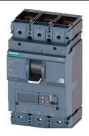
CIRCUIT BREAKER 3VA2 IEC FRAME 630 BREAKING CAPACITY CLASS M ICU=55KA @ 415 V 3-POLE, LINE PROTECTION ETU550, LSI, IN=400A OVERLOAD PROTECTION IR=160A ...400A SHORT CIRCUIT PROTECTION ISD=0,6..10X IN, II=1,5..15X IN NEUTRAL PROTECTION OPTIONAL WITH EXT. CT;UPTO 160% BUSBAR CONNECTION
