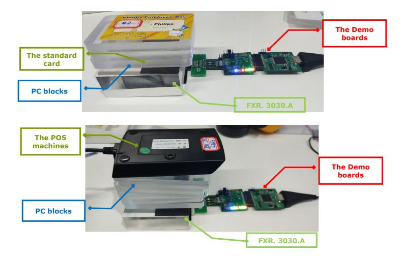
When the number of the PC material blocks are carefully adjusted until the reader can no longer read the sample, that's mean in this point the FXR.3030.A cannot establish communication with the standard card or the POS machine, the thickness of the PC material block is the maximum interrogation distance of them.
