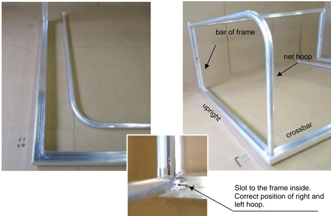
Fixing of net hoop at the top: Push nuts (position angle crossbar/upright) already provided in the upright below the slotted plate of the net hoop (see picture bottom left). Stick 2 washers DIN 9021, DIN 912,  $\text{\O} 7.4 \text{ mm}$  on 2 hexagon socket cylinder screws DIN 912, M6 x 20 and then screw the net hoop in the nuts (see picture bottom right and mid).
