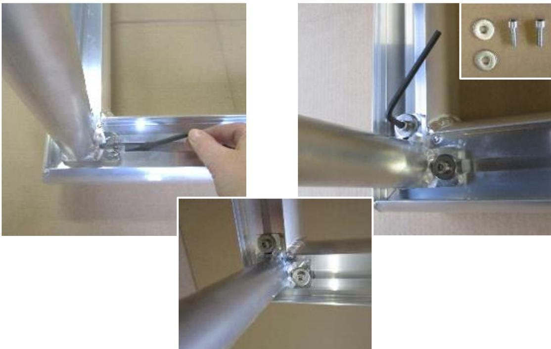
Fixing of net hoop at the bottom: At first erect the goal (see picture bottom left). Push the nut already provided in the ground frame angle below the slotted plate of the net hoop. Stick 1 washer DIN 9021, DIN 912,  $\text{\O} 7.4$  mm on 1 hexagon socket cylinder screw DIN 912, M6 x 20 which is then to be screwed in the nut to fix the net hoop (see picture bottom right).
