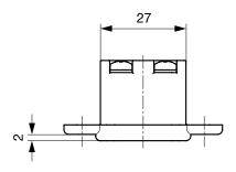
Protection class II, countersunk mounting holes, 40 mm distance, quick connect and solder terminals
