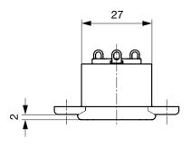
E: Quick-connect terminals 4.8x0.8 mm: 26.1 mm E: Quick-connect terminals 6.3x0.8 mm: 27.1 mm
